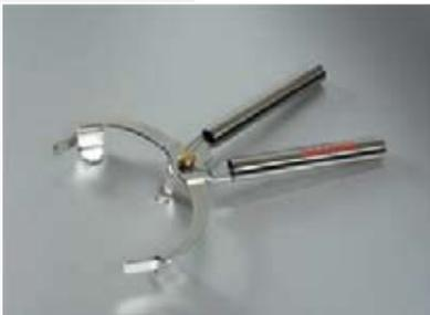
Gripper tools: The side openings in the rings allow you to grip below the base with optional tool and easily load and unload the high temperature furnace.
