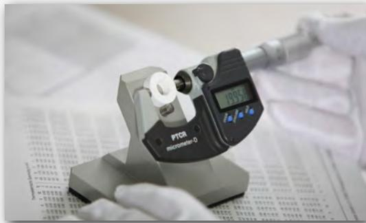
**Calibration** with PTCR (Pyrolytic Temperature Calibration Ring) simplifies calibration of the AUSTROMAT® 664 iSiC®. As this technique is not easy to analyze, DEKEMA naturally supports you by exactly evaluating the PTC ring. Satisfying our highly sophisticated customers with perfect tools, that's what DEKEMA® stands for.
